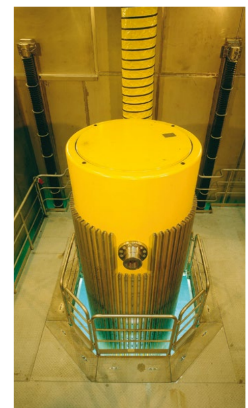
POLLUX®-type disposal container for salt formations
